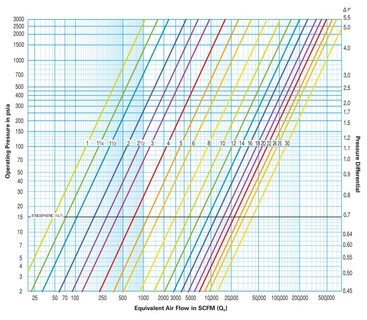
Actual Pressure Drop = Application's Equivalent Air Flow SCFM (Q<sub>c</sub>)
